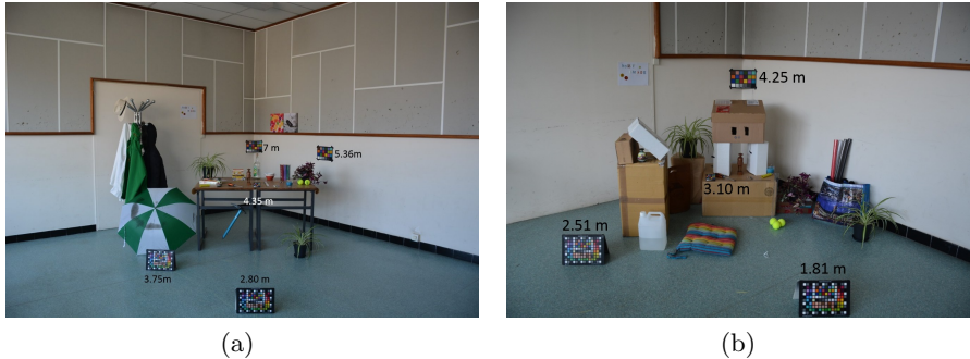
Fig. 1: Scene A (a) and Scene B (b). The distances of different MCCs to the camera are shown. The resolution of the image is 6000 \times 4000 .
