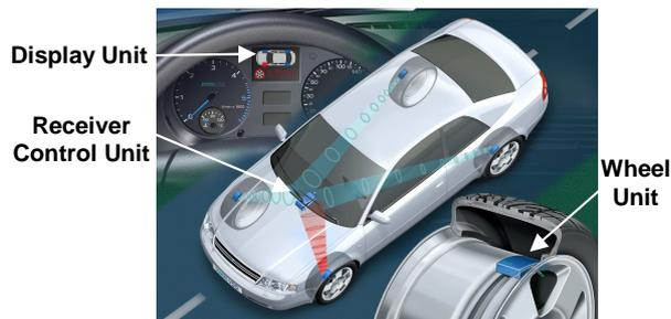
Fig. 1: Tire Pressure Monitoring System
