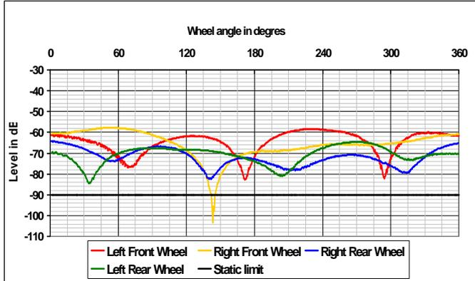
Fig. 2: field variation of TPMS (measured between the sensor in the wheel and the receiver) versus the angle of the wheel.
