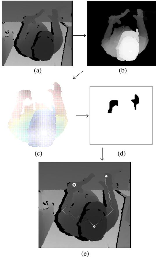
**Figure 2: Our hands-tracking method. (a): initial depth map, (b): upper body of the worker, (c): geodesic distances between each point of the upper body and the head (blue to red), (d): farthest upper body parts from the head, (e): head and hands locations with the shortest paths between the hands and the head**
