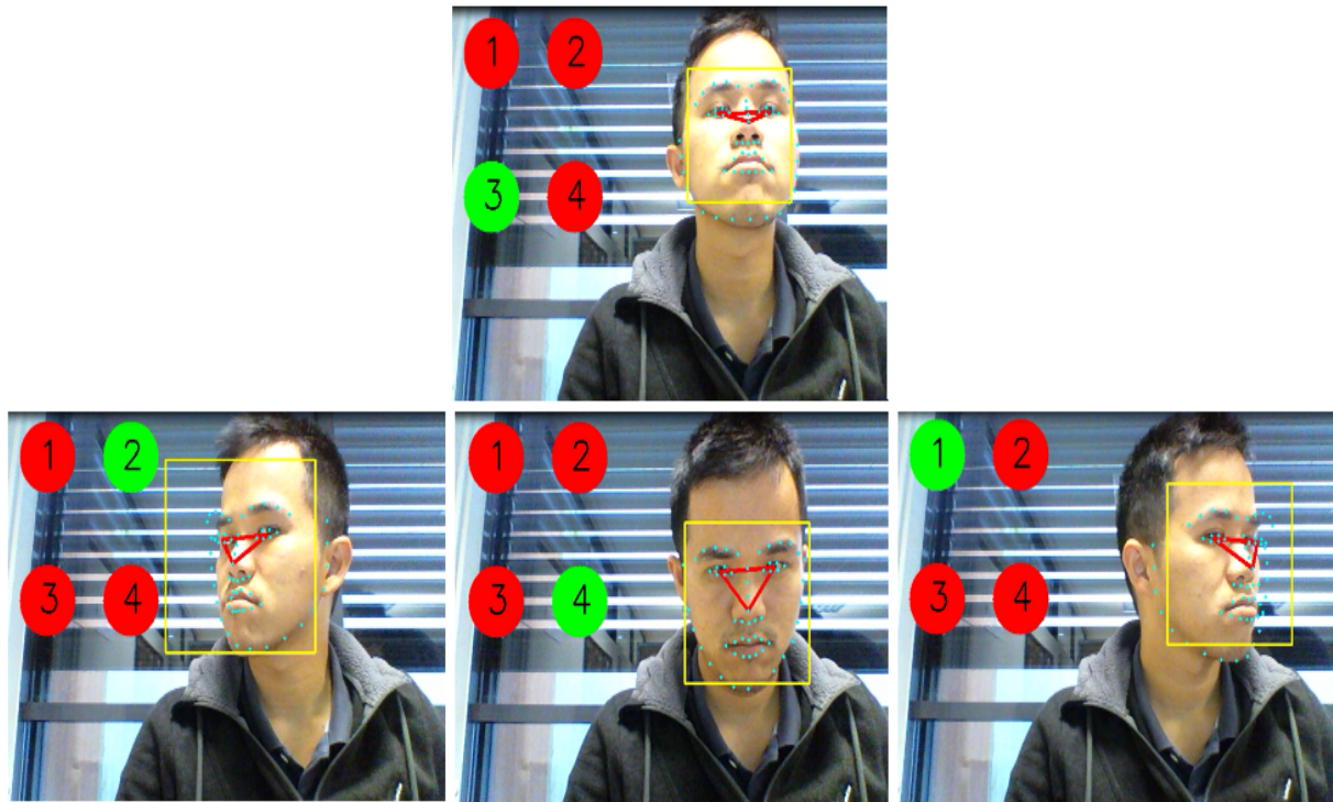
Figure 6 - Different state detection. The state is indicated by the number of the green circle. In state1 the student looks left; in state 2 he looks right; in state 3 he looks up; and in state 4 he is concentrated on the given task.
