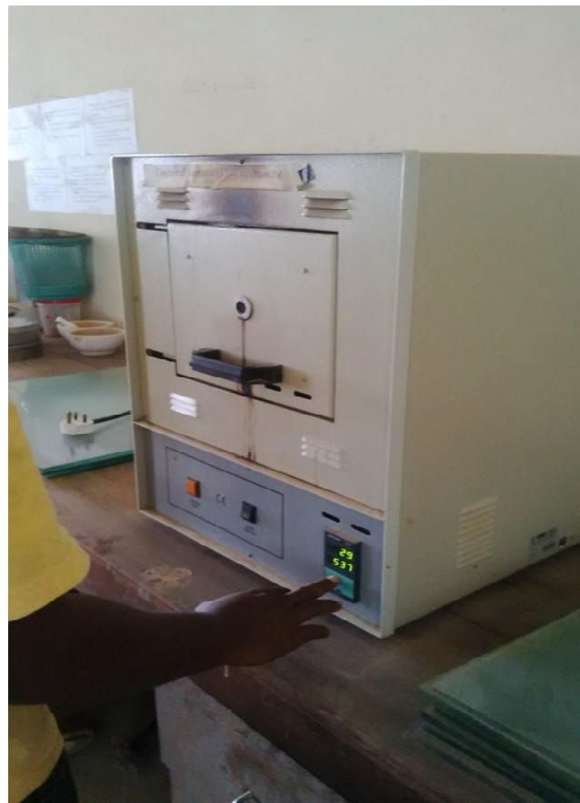
*Plate III. The furnace used for precipitation treatment.*
