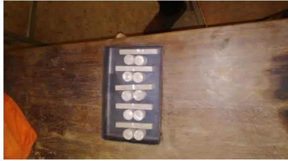
Plate II. Impact and hardness test specimens before being subjected to ageing process.
