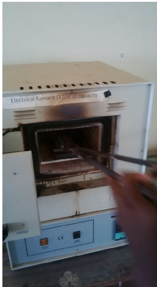
Plate IV. Removal of specimen after each hour of ageing time.
