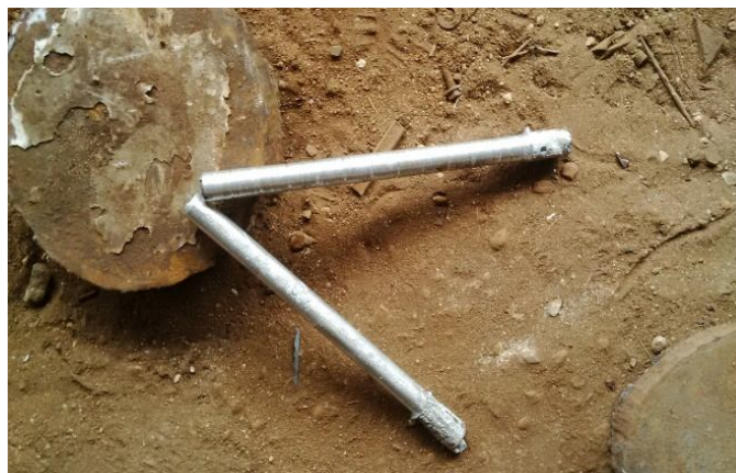
Plate I. Sample test bars of Al-2.00Mg-2.66Si Alloy.
