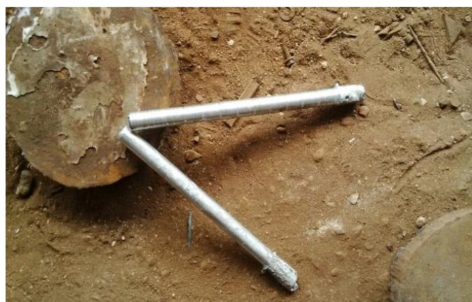
*Plate I. Sample test bars of Al-2.00Mg-2.66Si Alloy.*
