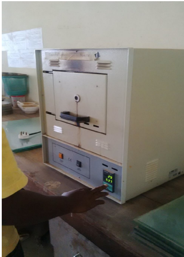
Plate III. The furnace used for precipitation treatment.
