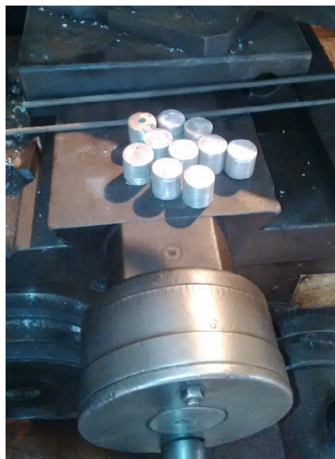
Plate V. Hardness specimen before undergoing hardness test.
