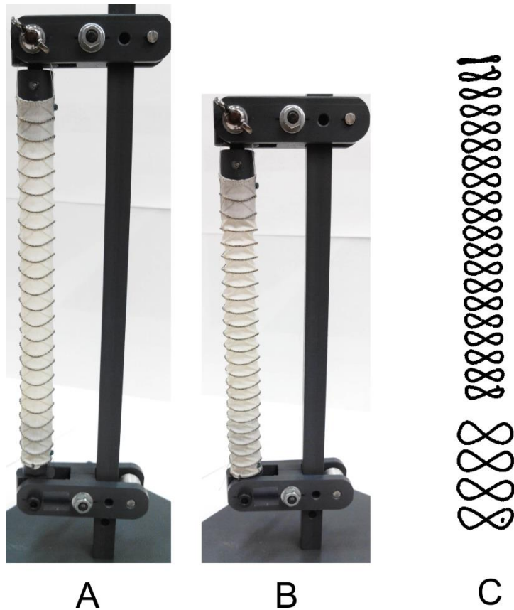
Figure 4. Experimental setup inserted in the microtomograph to derive the geometry of SG modules in stretched (A) and tension-free (B) states. Example of stent neutral axes extracted from microtomography scan images (C).
