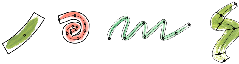
Fig. 1.6 Example spline strokes textured along a quad-strip defined from the curved stroke path.
