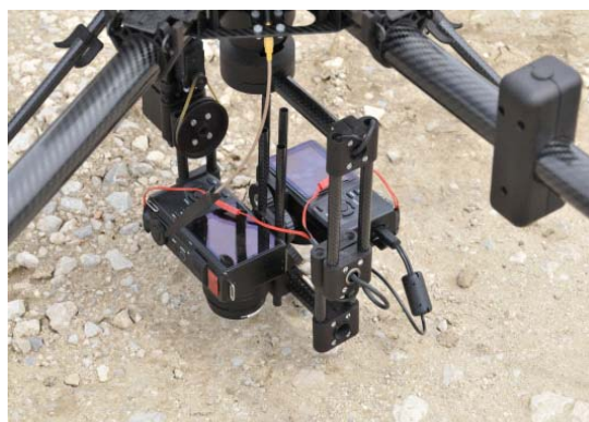
Figure 2. Two Sigma DP2 Merrill cameras mounted on UAV
