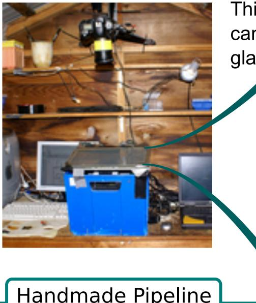
This typical setup for handmade painterly animation has a camera placed over a glass canvas to take snapshots. The glass is front- and backlit.
