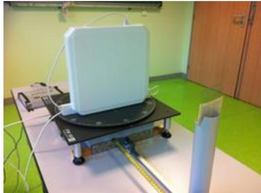
Fig. 7.b. Tag mounted on the sliding support.
