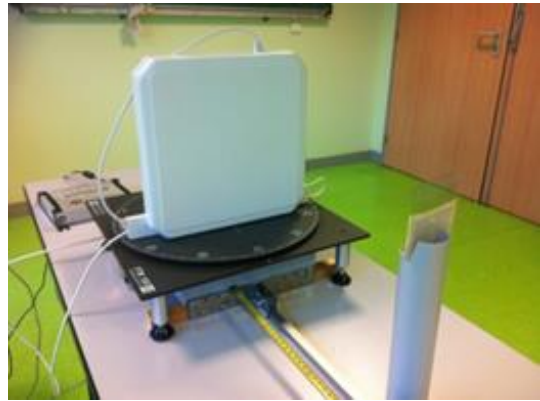
Fig. 7.b. Tag mounted on the sliding support.
