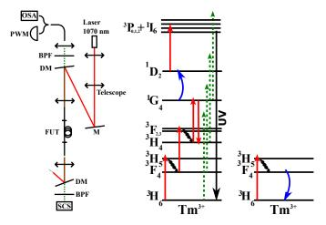
Figure 1: (Left): Experimental setup for PIA measurement. M: dielectric mirror, FUT: fiber under test, BPF: band pass filter, DM: dichroic mirror, OSA: optical spectrum analyzer, SCS: supercontinuum source, PWM: power meter. (Right): Energy level diagram of  $Tm^{3+}$ : red: pump induced transitions, blue: energy transfer, green:  $550 \ nm$  probe.
