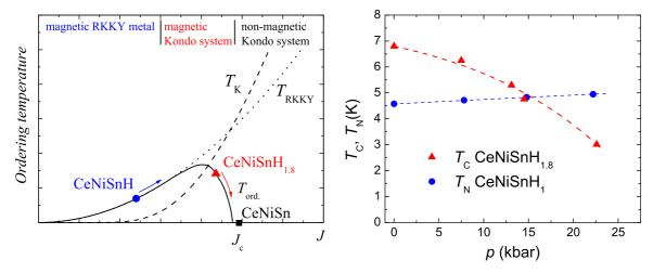
FIG. 12. Left: Schematic representation of Doniach's phase diagram indicating the relative position of the CeNiSnH $_x$  compounds (x = 0,1, and 1.8). Right: The pressure dependence of the Néel and Curie temperature of the H1 and H1.8 hydrides, respectively. Dotted lines are guides for the eyes.
