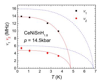
FIG. 4. Temperature dependence of the Larmor frequencies  $v_i$  at 14.5 kbar. The continuous (red) line represents the fit described in the text and the dotted (blue) lines show the  $v_i(T)$  dependency at ambient pressure.
