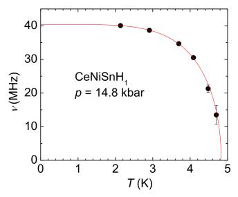
FIG. 9. Temperature dependence of the Larmor frequency  $\nu$ , for the P1 sample, at 14.8 kbar. The continuous (red) line is a fit of Eq. (2) to the  $\nu(T)$  data.
