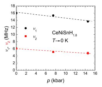
FIG. 5. Pressure dependence of  $\nu_1(T \to 0)$  and  $\nu_2(T \to 0)$ . Dotted lines are guides to the eye.
