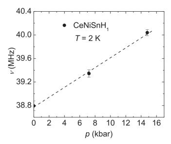
FIG. 10. Pressure dependence of the Larmor frequency  $\nu(T=2~{\rm K})$  for the P1 sample. The dotted line is a guide for the eye.
