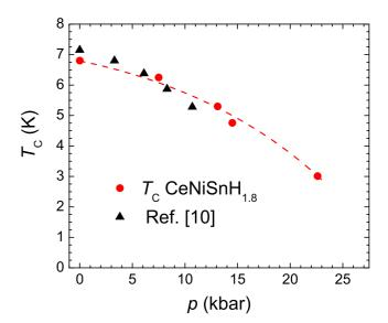
FIG. 6. Pressure dependence of the transition temperature  $T_C$  (red points) for CeNiSnH<sub>1.8</sub>. The triangles show results obtained from macroscopic measurements [10]. The dotted line is a guide for the eye.
