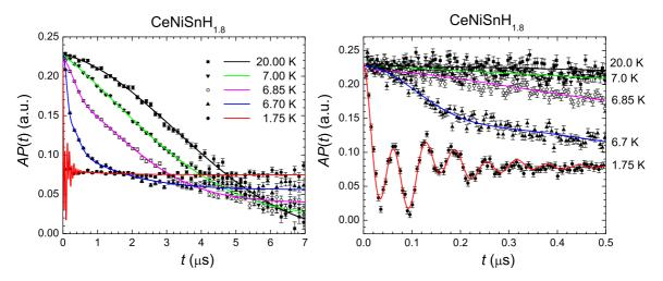
FIG. 1.  $\mu$ SR spectra recorded at selected temperatures above and below  $T_C$ . Left: long time scale; right: small time scale. Lines are fits of Eq. (1) to the data.
