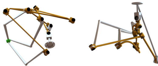
Fig. 4 Hand design for twist subspace, left; hand design for approximate trajectory synthesis, right.
