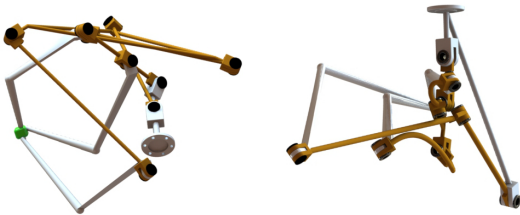
Fig. 4 Hand design for twist subspace, left; hand design for approximate trajectory synthesis, right.
