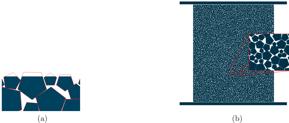
Figure 2: (a) Smoothing of pentagons in the contact boundary with walls. (b) Typical packing of 5000 regular pentagons used in compression simulations.
