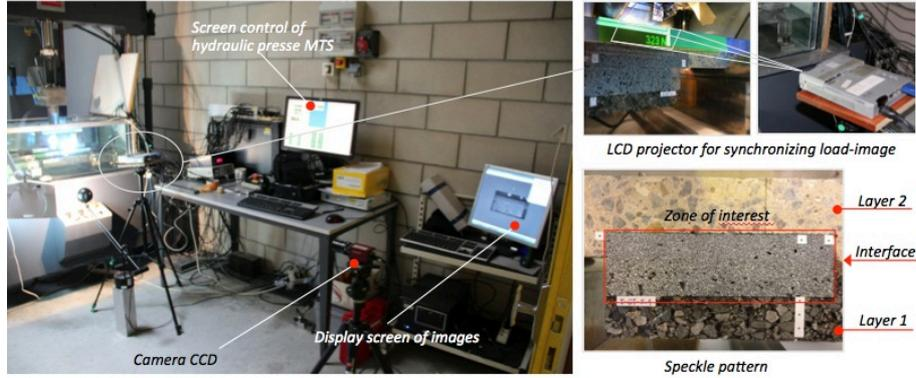
**Fig. 2** General description of the immersed 4PB equipment with DIC system
