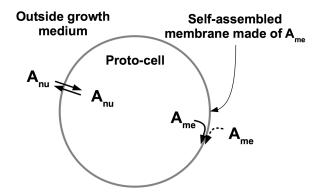
Fig. 1 Schematic of the protocell model. Some nutrient species  $(A_{\text{nu}} \in \mathcal{S}_{\text{nu}})$  flow across the semi-permeable membrane (e.g. by passive diffusion or active transport). The membrane results from the self-assembly of the membrane precursor  $A_{\text{me}}$ . The membrane surface area grows as the result of  $A_{\text{me}}$  unidirectional incorporation in the self-assembled membrane.
