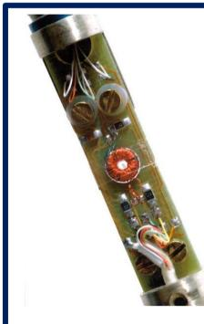
SQUID (Superconducting Quantum Interference Device) magnetometers are sensitive instruments which can track magnetic fields at a level of fT/Hz<sup>1/2</sup>, far beyond the sensitivity of fluxgate sensors, over a bandwidth of quasi dc – 10kHz. There are not sensitive to the absolute magnetic field, but just track changes. The length of time for which they track the field is limited by interference glitches. Periods of several days are usual in quiet conditions in a low noise environment.
