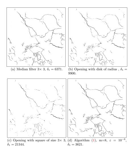
FIGURE 3.6. Comparison of the solutions computed with different filters, for a noise level equal to 0.05. Here  $\delta_1$  is the  $\ell^1$  norm of the difference between the ground truth and the solution, that is the number of pixels that are different.
