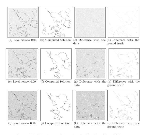
FIGURE 3.3. Noisy image, solution given by Algorithm (1) and difference with the ground truth, for different noise levels - m = 8,  $\varepsilon = 10^{-6}$  - The differences are presented as negative images for a better insight (white is equal to 0, black is maximum).
