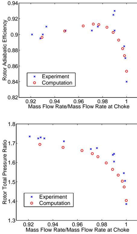
Figure 5. Comparison of Rotor Performance at Design Speed
