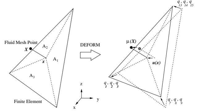
Figure 2. DEFORMATION TRACKING SYSTEM
