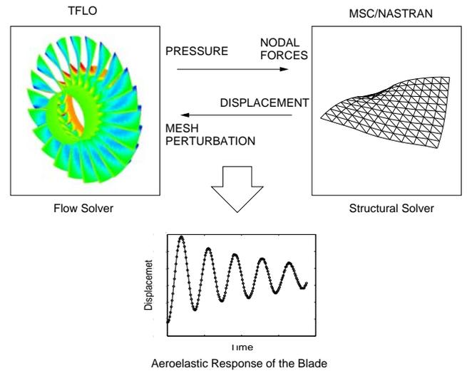
Figure 1. FLUID/STRUCTURE COUPLING
