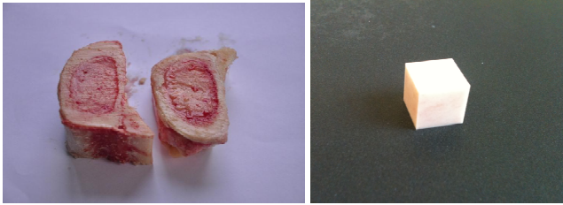
Figure 1: Beef cortical bone. Specimen before preparation (left) and after preparation (right) (cube with dimensions 0.01 \times 0.01 \times 0.01 \text{ m}^3 )
