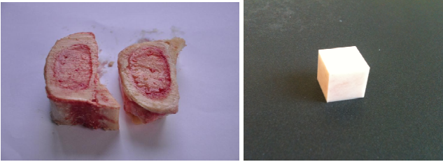
Figure 1: Beef cortical bone. Specimen before preparation (left) and after preparation (right) (cube with dimensions 0.01 \times 0.01 \times 0.01 m^3 )
