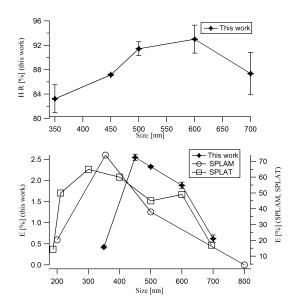
**Figure 6.** The scattering efficiency and the hit rate as a function of the size of various PSL particles (350, 450, 500, 600, and 700 nm) at a particle number concentration of 20 cm<sup>-3</sup>. The SPLAT and SPLAM scattering detection efficiency results are given for comparison purpose.
