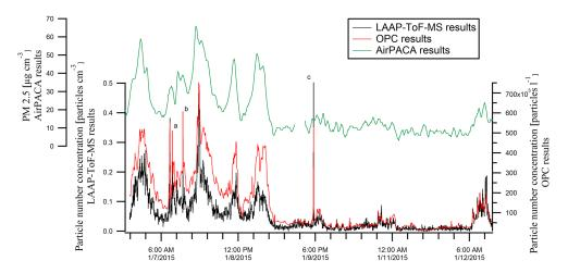
**Figure 4.** The total particle number concentration detected by LAAP-ToF-MS and OPC as a function of time; indicated are peaks corresponding to smoking events (**a** and **b**) and to generation of TiO<sub>2</sub> (**c**). The total PM<sub>2.5</sub> results according to Air PACA are depicted in green.
