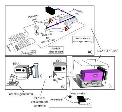
**Figure 1.** (a) Schematic diagram of the working principle of LAAP-ToF-MS, (b–c) Experimental configuration aimed to investigate the influence of particle density, size effect and detection efficiency, and (c–d) Experimental configuration for aerosol particle measurement.
