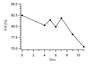
**Figure 3.** The influence of the ArF gas life time on the evolution of the laser hit rate (HR) over the time.
