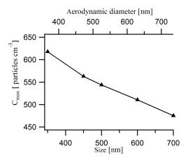
**Figure 12.** Variation of  $C_{\text{max}}$  for particles with different aerodynamic diameters.
