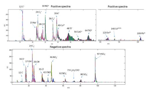
Figure 5. The standard deviation of all positive and negative ion mass spectra.
