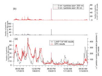
**Figure 14.** (a) The number of particles sizes between 200–300 nm detected by the LAAP-ToF-MS every 50 min and the number concentration detected every 5 min by the OPC for the particles sizes 250–300 nm. (b) the number of particles having a size between 0–200 and 0–80 nm detected by the LAAP-ToF-MS every 5 min.
