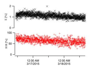
**Figure 2.** Repeatability of the scattering efficiency (E) and the hit rate (HR), during a time period of 53 h.
