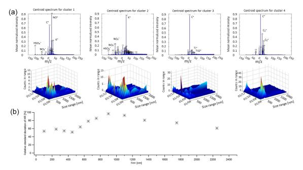
**Figure 9. (a)** Different clusters of particles and their evolution during the measurements in different size range between 10 and 2500 nm. **(b)** The standard deviation of the total hit rate calculated every 5 min during the measurements for each size range.
