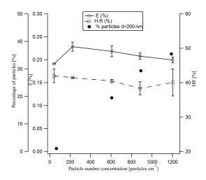
**Figure 13.** The hit rate and the scattering efficiency of 450 nm ferric sulfate particles as a function of the particle number concentration and the percentage of the particles having a size lower than 200 nm for different concentrations of generated particles.
