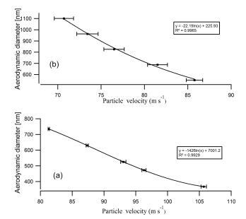
**Figure 11.** Plot of aerodynamic particle size versus particle velocity for (a) PSL particles and (b) ammonium nitrate particles.
