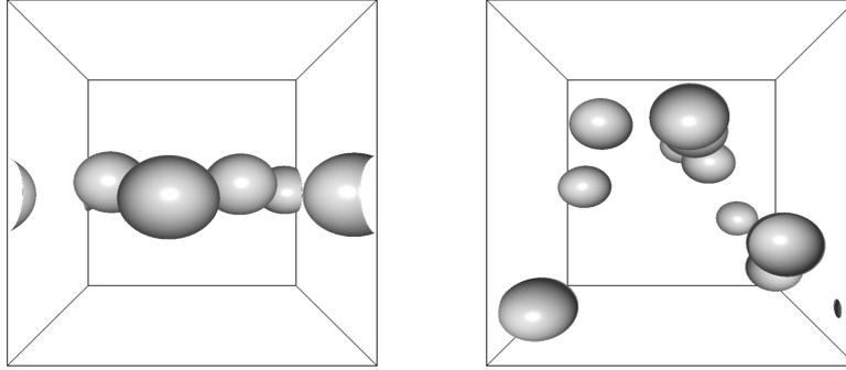
**Figure 20.** Influence of the number of free bubbles on their spatial distribution within a periodic unit cell: typical instantaneous snapshots for  $N_b = 4$  (left) and  $N_b = 8$  (right), for case E1 at  $\phi = 3.8$  %.
