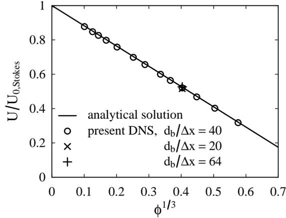
**Figure 2.** Steady drift velocity of an ordered array of spherical bubbles normalized by that of an isolated bubble in the Stokes flow regime (case S0) as a function of volume fraction, compared to the analytical solution of Sangani (1987). The effect of resolution is shown for  $\phi^{1/3} = 0.4$  ( $d_b$  is the bubble volume-equivalent diameter,  $\Delta x$  the grid spacing).
