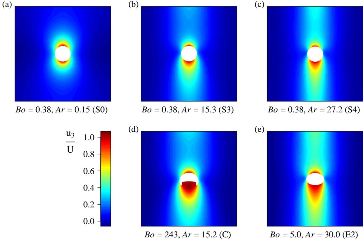
**Figure 5.** Vertical component of the liquid velocity normalized by the bubble drift velocity in a vertical symmetry plane passing through the center of a bubble in an ordered array configuration at  $\phi = 0.2\%$ . Gravity is pointing downward ( $\mathbf{g} = -g\mathbf{e}_3$ ). Increasing Archimedes numbers from left to right, and increasing Bond numbers from top to bottom.
