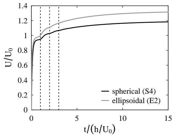
**Figure 6.** Time signal of the normalized drift velocity of an ordered array of bubbles at small volume fraction ( $\phi = 0.1\%$ ). The dashed vertical lines denote  $t = nh/U_0$ , the characteristic times at which the bubbles enter into the wake of their  $n^{\text{th}}$  preceding neighbour. For clarity only short times are shown (the steady-state is reached for  $t \approx 50h/U_0$ ).
