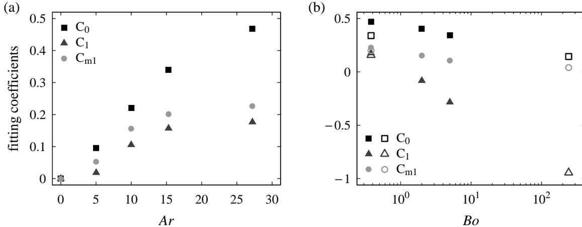
**Figure 9.** Fitted coefficients for  $U(\phi)/U_0$  as given by (24): (a) as a function of the Archimedes number for  $Bo = 0.38$ , (b) as a function of the Bond number for  $Ar \approx 15$  (open symbols) and for  $Ar \approx 30$  (filled symbols). The coefficients are obtained by least-squares fits of DNS and isolated-bubble data.
