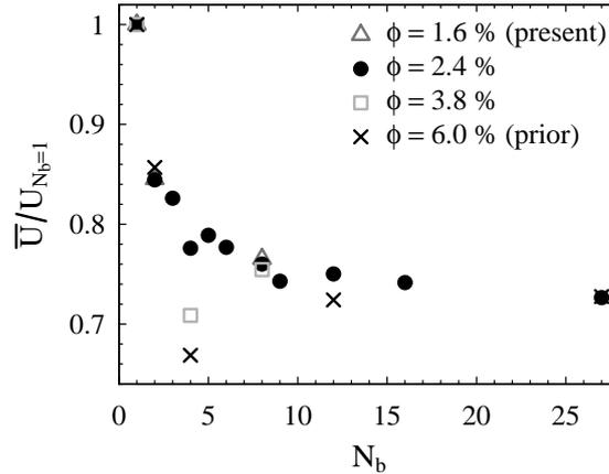
**Figure 19.** Influence of the number of bubbles on the average bubbles drift velocity for various volume fractions. The drift velocity is normalized by that obtained in the ordered configuration ( $N_b = 1$ ). Symbols other than crosses: present DNS for case E1 ( $Ar = 29.9$ ,  $Bo = 2.0$ ). Crosses: prior DNS of Bunner and Tryggvason (2002) for a comparable flow regime ( $Ar = 29.7$ ,  $Bo = 0.98$ ).
