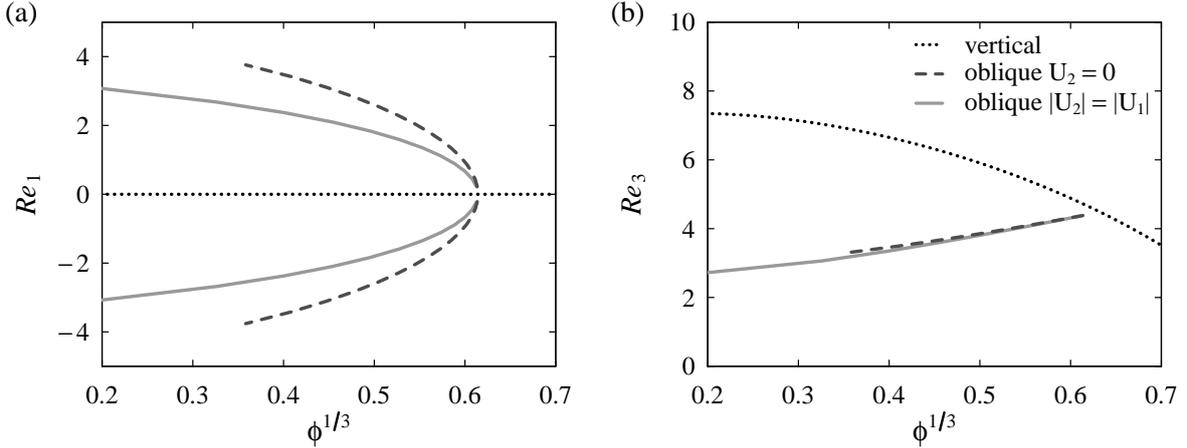
**Figure 13.** Subset of analytical solutions obtained from solving (55) for  $Ar = 20$  and  $\rho_d/\rho_c = \mu_d/\mu_c = 0$ : bubble drift velocity horizontal (a) and vertical (b) components, given as Reynolds numbers  $Re_i = U_i \rho_c d_b / \mu_c$ , as a function of volume fraction. Gravity is pointing in the  $-\mathbf{e}_3$  direction.  $\cdots$ : vertical rise ( $U_1 = U_2 = 0$ );  $---$ : oblique rise with  $U_2 = 0$ ;  $—$ : oblique rise with  $|U_2| = |U_1|$ .
