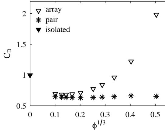
**Figure 7.** Drag coefficient as a function of volume fraction for case S4.  $\nabla$ : ordered array;  $*$ : trailing bubble of a vertically-aligned pair within the same conditions (Reynolds number, separation distance), from Hallez and Legendre (2011);  $\blacktriangledown$ : isolated bubble, estimated from Mei, Klausner, and Lawrence (1994).
