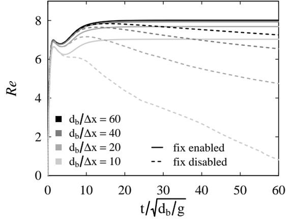
**Figure 24.** Effects of resolution and of volume conservation enforcement on the rise of an ordered array of strongly deformed bubbles (case C at  $\phi = 1.6\%$  with  $\rho_d/\rho_c = 0.1$  and  $\mu_d/\mu_c = 0.1$ ).
