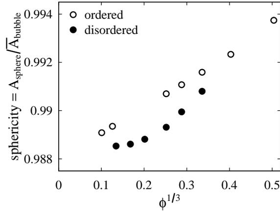
**Figure 22.** Influence of volume fraction on the bubbles sphericity in ordered (open circles) and disordered (filled circles) configurations in case E1. The sphericity is defined as the ratio between the total surface areas of a set of  $N_b$  volume-equivalent spheres and that of the bubbles.
