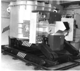
Fig. 2: Magnetodynamic mixer-batcher for overheating and pouring of cast iron and steel
