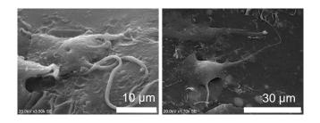
**Figure 10.**NHOst cells on a scaffold of 1HCPS after 20 days of culture. NHOst cells can be seen attached to the surface with numerous projections.
