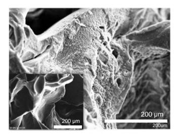
**Figure 4.** Addition of ammonia carbonate to sugar porogen forms rough scaffold surface. Inset: surface without the addition  $(NH_4)_2CO_3$ .
