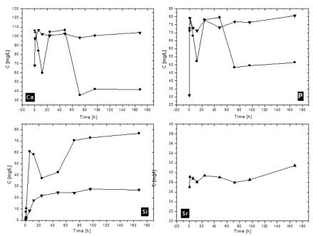
**Figure 5.** Inductively coupled plasma analysis of the evolution of  $Ca^{2+}$ ,  $Si^{4+}$ ,  $PO_4^{3-}$  and  $Sr^{2+}$  ions (mg L<sup>-1</sup>) in DMEM. Dots, 1HCPP; triangles, 1HCPSP.
