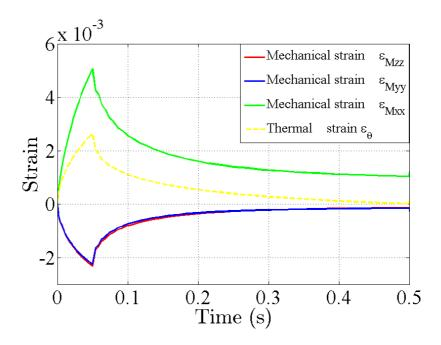
Figure 10: Predicted contributions of the thermal and mechanical parts to the in-plane and out-of-plane normal strains
