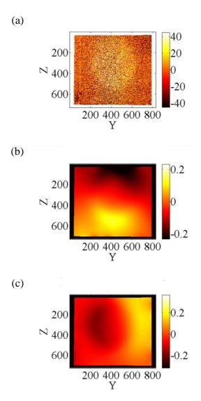
Figure 8: (a) Correlation residual map expressed in grey levels (dynamic range of the picture: 4080 grey levels). Displacement fields along Y (b) and Z (c) axes (expressed in pixel) between pictures taken just before starting a laser pulse and at the end of the laser pulse
