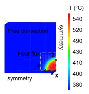
Figure 4: Illustration of the symmetric thermal boundary conditions (with the identified super-Gaussian) applied to the 3D model. The dotted box represents the zone of finer mesh.
