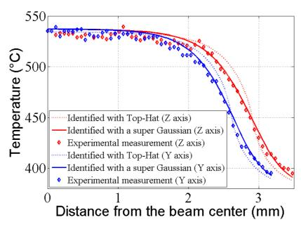
Figure 6: Averaged experimentally measured (IR) and identified temperature profiles along the vertical (Z, red) and horizontal directions (Y, blue) at the end of a laser shock. The dashed line corresponds to the prediction with a top-hat power density function, and the solid line with a super-Gaussian
