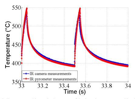
Figure 7: Temperature history in the centre of the laser beam measured by the largeband pyrometers and IR thermography
