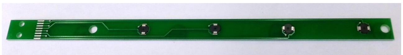
Fig. 7. In-house developed sampler: L \times W \times H = 300 \times 15 \times 3 mm.
