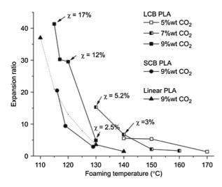
**Fig. 4.** Expansion ratio and bulk crystallinity of PLA foams as a function of processing temperature and CO<sub>2</sub> concentration by Wang et al. [24]. (Reprinted with permission from [24], © 2012 Elsevier).
