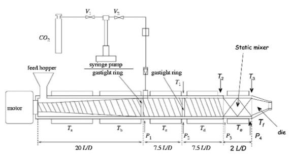
Fig. 1. Schematic of the single-screw extruder used by Fages et al. [15,19–23]. (Reprinted with permission from [15], © 2014 Elsevier).
