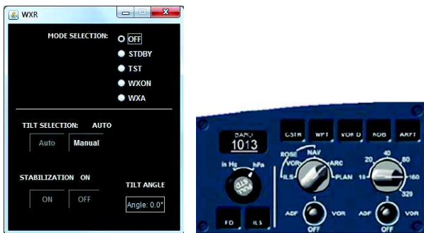
Figure 3 - Image of a) the weather radar control panel b) of the radar display manipulation
