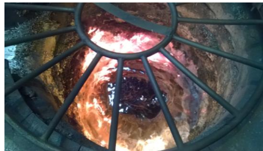
Fig. 4: Free surface of industrial furnace. Dome with small fluctuation (E2).
