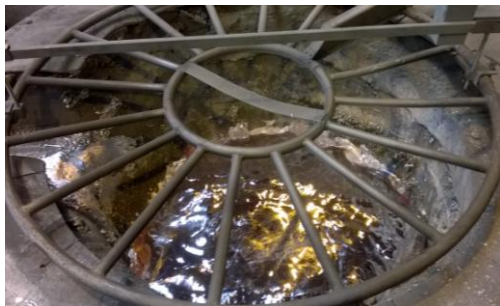
Fig. 3: Free surface of industrial induction furnace. Dome with large fluctuation (E1).
