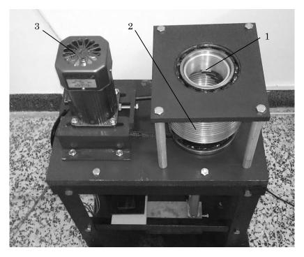
Figure 2. Experimental setup of magnetic stirrer. 1-permanent magnets, 2-stirrer, 3-motor.
