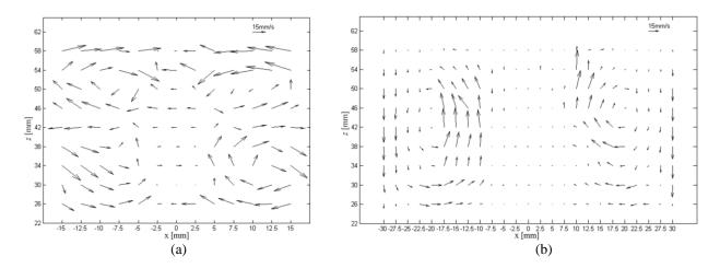
Figure 3. Meridian vector velocity fields at the cross-section y = 0 indicating the flow patterns of meridian (a) secondary flow (D/H = 1) and (b) global axial flow (D/H = 1.75) driven by an electromagnetic stirrer.
