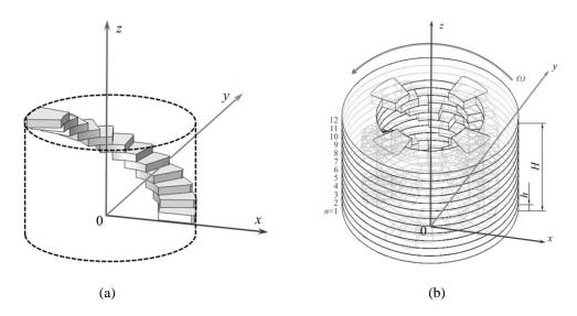
Figure 1. A helical permanent magnet and its construction.
