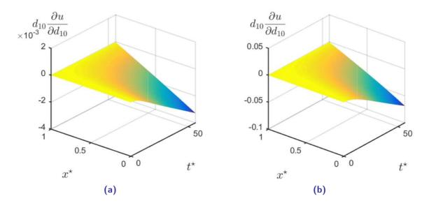
**Figure 12.** Sensitivity coefficient of parameter  $k_0$  for experimental conditions  $\pi$  where  $\Psi$  reaches its minimal value (a)  $\left(\frac{2\pi}{\omega_1}=3.3 \text{ days}, \frac{2\pi}{\omega_2}=495 \text{ days}, N=3\right)$  and for the ODE conditions (b)  $\left(\frac{2\pi}{\omega_1^\circ}=78.1 \text{ days}, \frac{2\pi}{\omega_2^\circ}=20.9 \text{ days}, N^\circ=1\right)$ .
