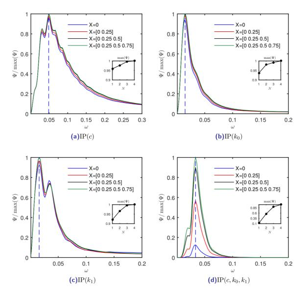
**Figure 4.** D-optimum criterion  $\Psi$  as a function of N, X and  $\omega$  for the 4 different experiments  $(A = A^{\circ} = 1)$ .
