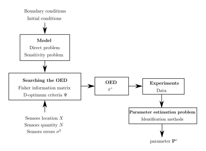
Figure 1. Process of searching the Optimal Experiment Design.
