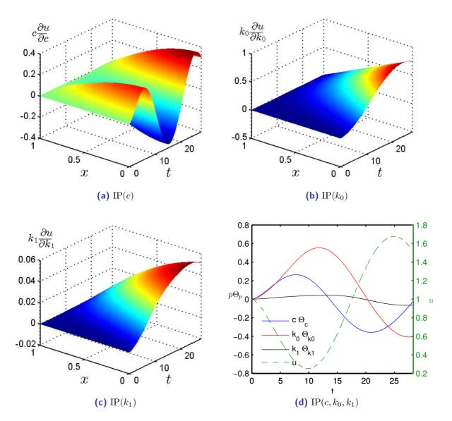
**Figure 5.** Sensitivity coefficient of parameters for the four different experiments  $(N = N^{\circ} = 1)$ .
