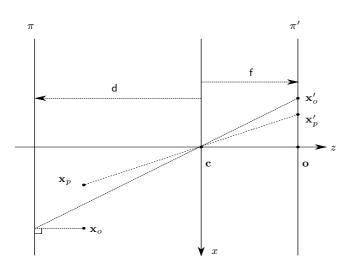
Fig. 1 Orthographic projection:  $\mathbf{x}_o$  is conjugate to  $\mathbf{x}'_o$ . Perspective projection:  $\mathbf{x}_p$  is conjugate to  $\mathbf{x}'_p$ .
