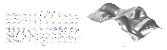
Fig. 4 (a) Gradient field estimated via photometric stereo. (b) Integration using a periodic boundary condition [19]. The depth is exactly the same on the left and right edges, i.e. on the cheek and on the nose, which much distorts the 3D-reconstruction.
