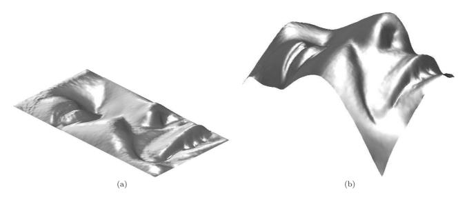
Fig. 5 (a) Integration of the gradient field of Fig. 4-a using the homogeneous Dirichlet boundary condition z = 0: since this is clearly false, the 3D-reconstruction is much distorted. (b) Integration using the (Neumann) natural boundary condition [48]. The natural boundary condition provides much more realistic results.
