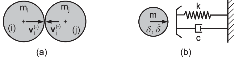
Fig. 3 (a) Contact between two rigid spheres; (b) Equivalent system
