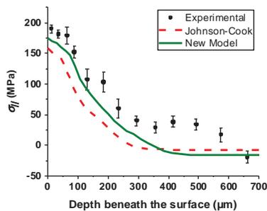
Fig. 4. Experimental and predicted residual stresses in cutting direction ( $\sigma_y$ ).
