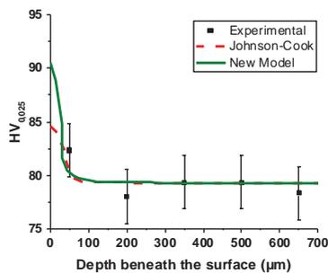
Fig. 3. Experimental and predicted Vickers micro hardness ( $HV_{0.025}$ )
