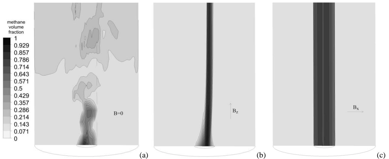
Fig. 4: Methane volume fraction instantaneous distributions in vertical cross-section of CBR inlet zone: (a)  $t = 40$  s,  $B=0$ ; (b)  $t = 13.5$  s,  $B_z = 0.5$  T (“switched on” for  $t = 10$ – $13.5$  s); (c)  $t = 20$  s,  $B_x = 0.5$  T (“switched on” for  $t = 10$ – $20$  s).
