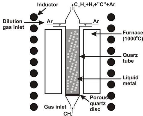
Fig. 1: Liquid metal bubble column for H<sub>2</sub> production without CO<sub>2</sub> emission.
