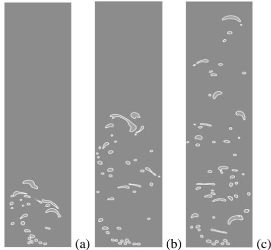
Fig. 3. Randomly generated bubbles in rectangular column  $L_x = 0.5 \text{ m}$ ,  $L_y = 2.5 \text{ m}$ :  $\rho_l/\rho_g = 1000$ ;  $\nu_l/\nu_g = 100$ : (a)  $t = 21.5 \text{ s}$ ; (b)  $t = 48.0 \text{ s}$ ; (c)  $t = 90.0 \text{ s}$ .
