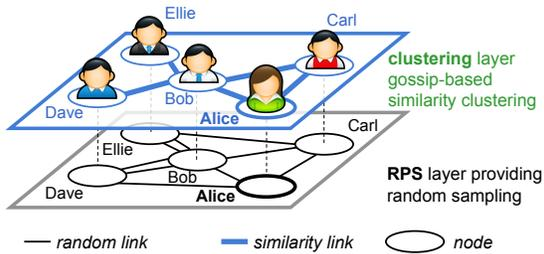
FIGURE 1 – Overlay Architecture
