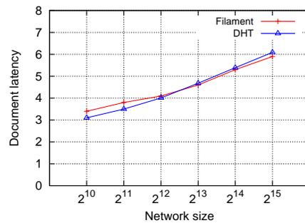
FIGURE 8 – Filament vs DHT based on document latency
