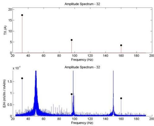
**Figure 2: Top: amplitude spectrum of the transmitted current. Bottom: amplitude spectrum of the recorded electric field. Please note the high level of anthropic noise (50Hz and harmonics), stronger than the recorded electric field at the CSEM frequency.**
