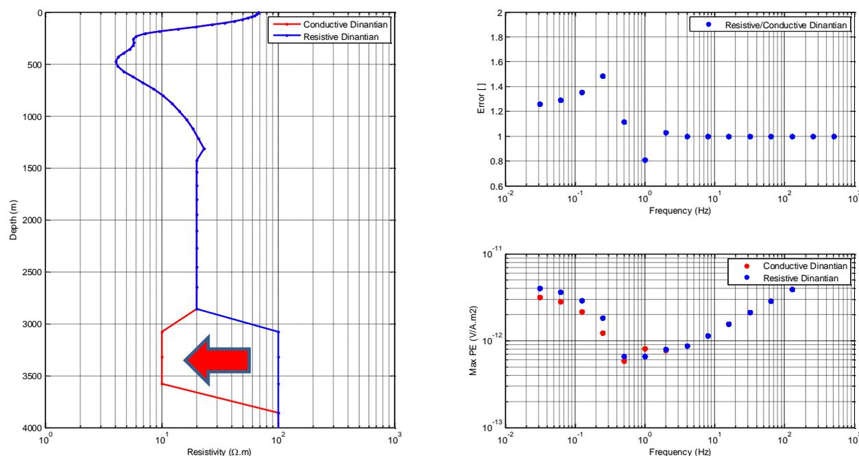
**Figure 8: Left: Resistivity model for a fissured (red) and intact (blue) limestone reservoir. Right: amplitude (bottom) and relative change (top) of the maximum axis of the polarization ellipse of the horizontal electric field 10km way from the CSEM source as a function of the CSEM source frequency.**
