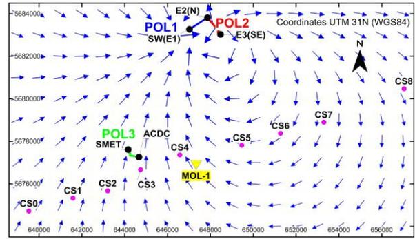
**Figure 1: CSEM/MT survey layout. CS0 to CS8 MT/CS stations. Location of the 3 dipoles (polarizations) used for current injection with electric field (in-phase) distribution at frequency 0.125 Hz in a 50  $\Omega$ m homogeneous medium drawn for POL1 only. The location of the new deep geothermal exploration well MOL-1 is represented by the yellow triangle.**
