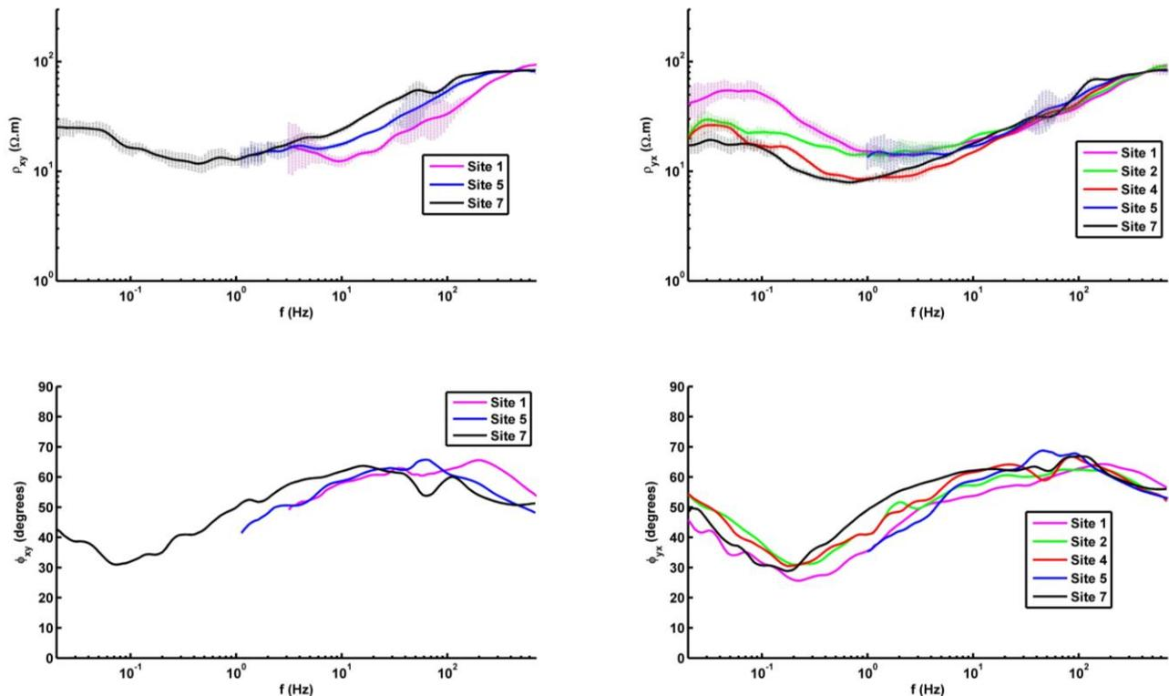
**Figure 3: Remaining MT soundings apparent resistivity (upper panel) and phase (lower panel) for sites 1,2, 4, 5 and 7. Left panel, top : apparent resistivity xy ( $\Omega\cdot\text{m}$ ), bottom : apparent phase xy (degrees). Right panel, top : apparent resistivity yx ( $\Omega\cdot\text{m}$ ), bottom : apparent phase yx (degrees). Error bars are shown on the resistivity curves as vertical dashed lines.**
