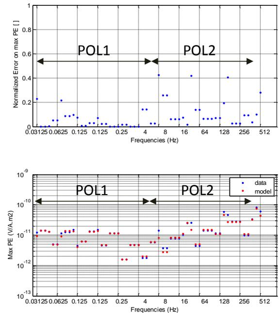
**Figure 4: Left: 1-D inversion (red) resistivity profile obtained from the smooth inversion of the CSEM data transmitted at 0.03125, 0.0625, 0.125, 0.25, 4, 8, 16, 32, 64, 128, 256, 512 Hz and both polarizations and recorded at stations 00, 01, 02, 03, 06 and 07. Top right: relative misfit between the modelled and observed CSEM data. Bottom right: observed (blue) versus modelled (red) maximum axis of the polarization ellipse of the horizontal electric field.**
