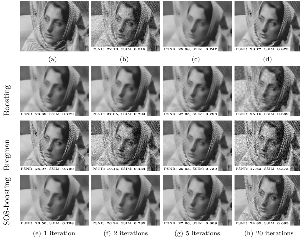
FIG. 16. (a) Image x_0 with moderate patch redundancy. (b) Noisy version y = x_0 + w . (c) Non-local means \hat{x}(y) with h = 5.5 . (d) Covariant re-fitting \mathcal{R}_{\hat{x}}(y) . (e,f,g,h) From top to bottom, boosting [48, 4], Bregman iterations [5] and SOS-boosting [38] at respectively 1, 2, 5 and 20 iterations.
