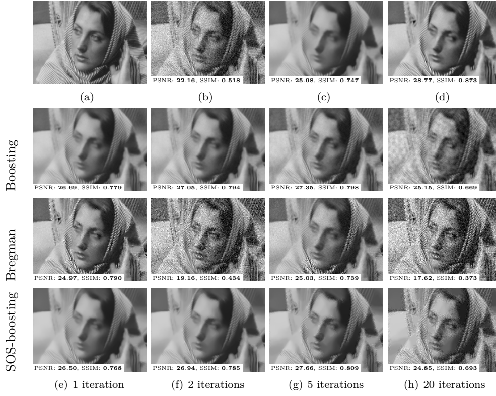
FIG. 16. (a) Image x_0 with moderate patch redundancy. (b) Noisy version y = x_0 + w . (c) Non-local means \hat{x}(y) with h = 5.5 . (d) Covariant re-fitting \mathcal{R}_{\hat{x}}(y) . (e,f,g,h) From top to bottom, boosting [47, 4], Bregman iterations [5] and SOS-boosting [37] at respectively 1, 2, 5 and 20 iterations.
