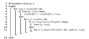
Fig. 3. Controlled Gossip Algorithm
