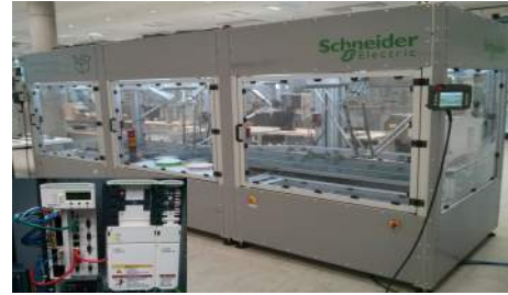
Fig. 7. Demonstrator with three robots and two parallel conveyors.
