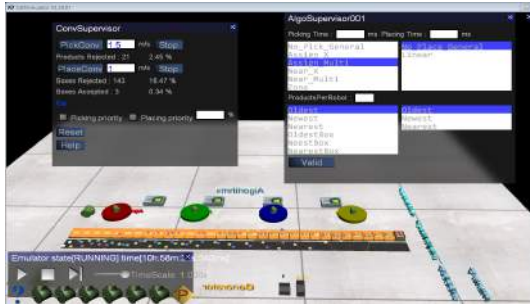
Fig. 5. Simulation example with four robots and two conveyors co-current with the DownToUp collaborative strategy.
