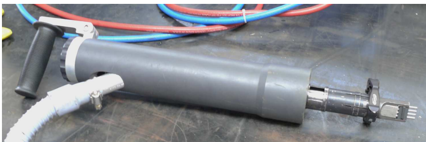
Figure 7: High frequency hammer peening tool used.
