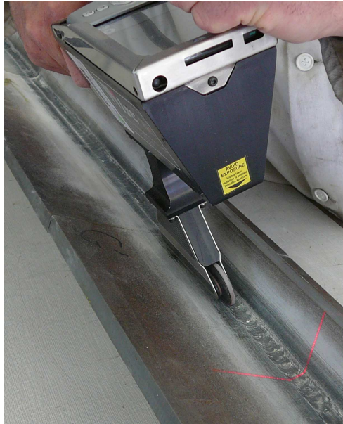
Figure 2: Laser triangulation dimensional analysis (WISC process).
