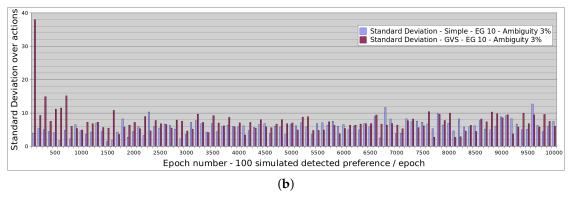
**Figure 6.** Simulated results comparing the GVS algorithm with a simple method using an epsilon greedy mechanism with  $\epsilon=10$  in the action selection process and with an ambiguity of 3% in users feedback. (a) the number of negative actions in each epoch; (b) the standard deviation between the number of times each action was used during an epoch.
