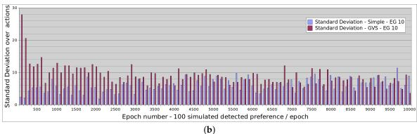
**Figure 5.** Simulated results comparing the GVS algorithm with a simple method using an epsilon greedy mechanism with  $\epsilon = 10$  in the action selection process. (a) the number of negative actions in each epoch; (b) the standard deviation between the number of times each action was used during an epoch.
