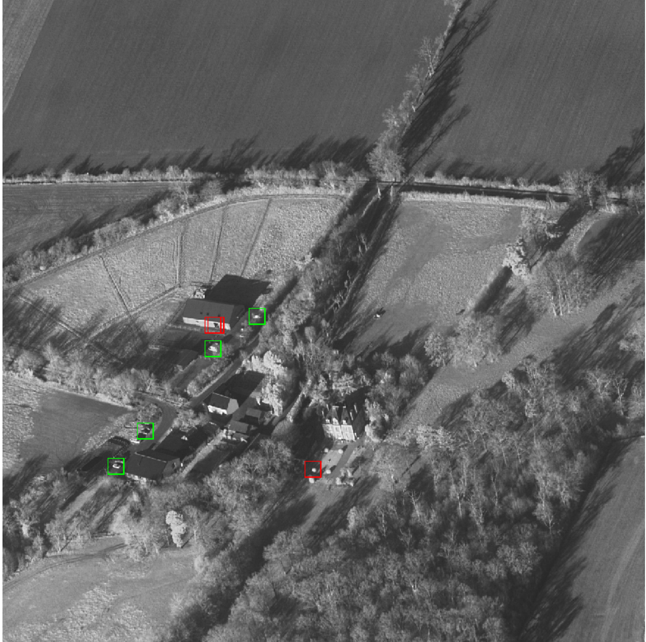
Fig. 7. This image is representative of a situation where the vehicles may be occluded behind vegetation elements. Here, we show that the correctly detected vehicles may be hardly recognizable for an untrained eye. Besides, we show that, although the image is highly textured, LR-CNN only outputs a very small amount of false detections - only three in this case.
