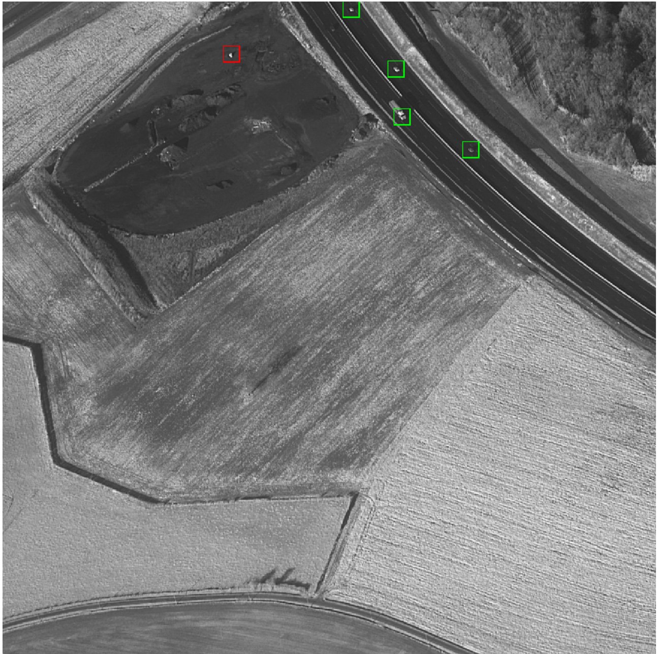
Fig. 6. This figure is representative of contexts where the vehicles are relatively easy to recognize, yet the background may be very textured in some parts of the image. We show that our network applied in a sliding window manner achieves detecting all the vehicles, except for one. Besides, the vehicle that is not detected is very dark, on a very dark background (the road): even the human eye has considerable difficulties detecting this target. It is also worth noticing that our model only outputs one false alarm on this image. This salient object is quite difficult to apprehend, and could easily be mistaken for a vehicle by a human eye.
