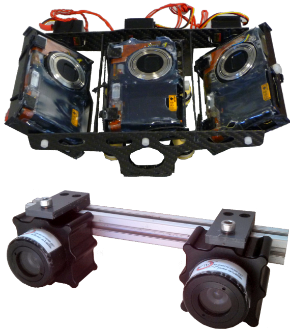
Figure 3: The developed payloads. Top: the tri-camera sensor, used on the Faucon Noir UAV. Bottom: the binocular stereoscopic rig, currently used on an underwater robot (sealed housings can be removed when the rig is used on a flying vehicle).
